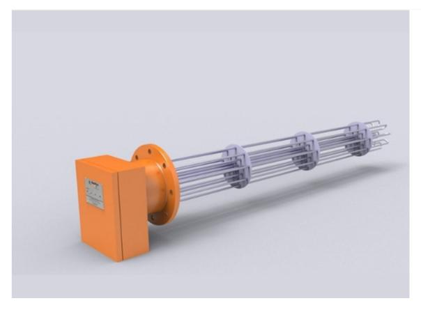
Immersion heaters are amongst the most popular heaters owing to wide customization, easier installation and operations in stringent environment. Made by brazing or welding flange with several hairpin elements or bulge tubular elements, these are designed for heating chemical, petroleum and water based applications specially heat transfer fluids, medium and lightweight oils and water in tanks and pressure vessels.
